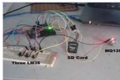
(b): SD card as mobile data Logger
