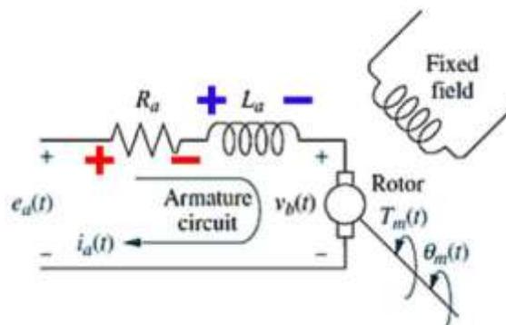
Fig.4. Circuit of service motor
