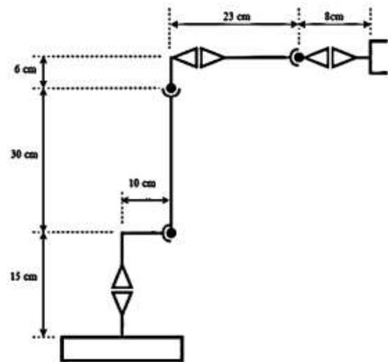
Fig.2. Symbolic structure of a RAMIS link length, the attached frames to the joints and the operational axis which is along the Z axis.
